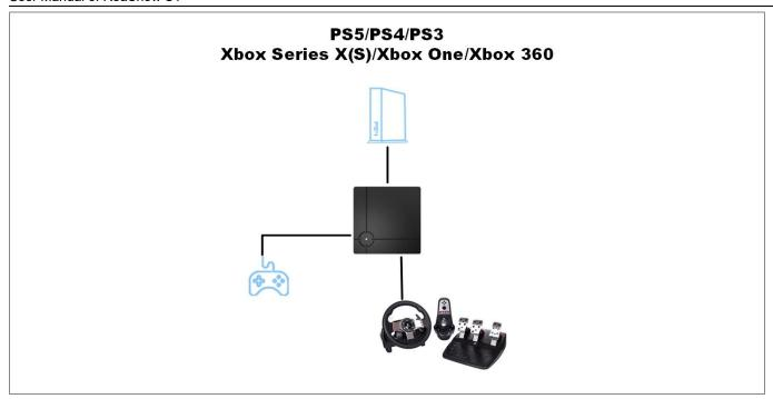
Firstly, connect the original controller (USB 1) and the wheel (USB 2 or 3) to ReaSnow S1, and then connect ReaSnow S1 to console.
